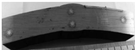
Figure 2. Sampling regions for chemical composition using optical emission spectroscopy.
