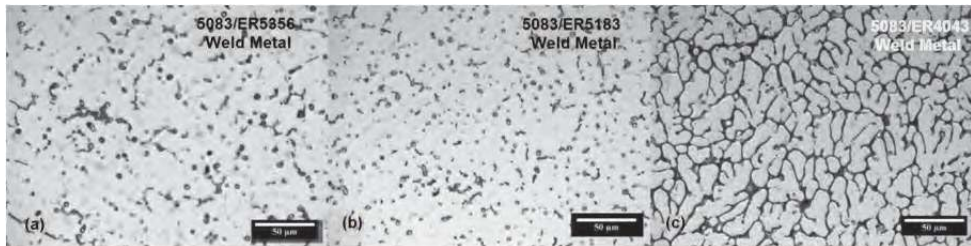
Fig. 15. Typical micrographs of (a) 5083/ER5356; (b) 5083/ER5183; and (c) 5083/ER4043 weld metal.
