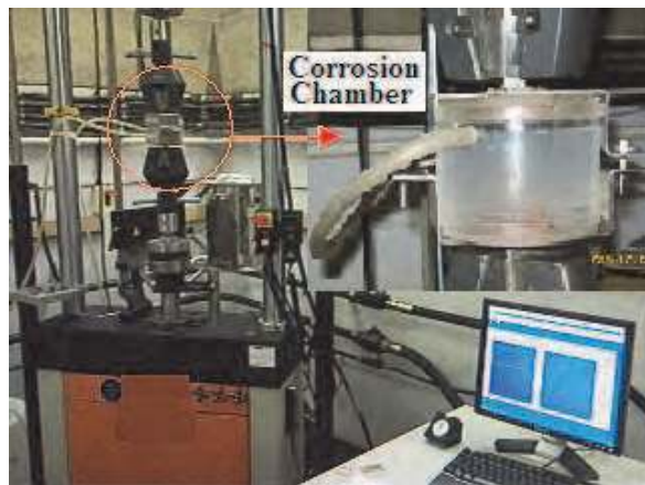
Fig. 10. The experimental set-up used for corrosion fatigue testing in a NaCl solution.
