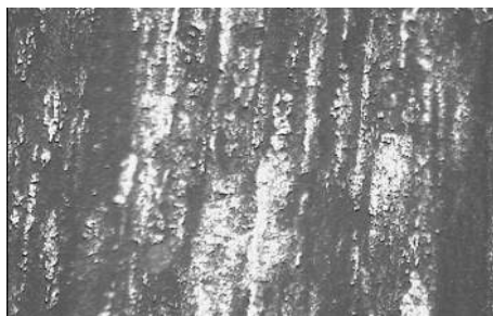
Figure 4 (a): -Mild steel sample blank kept in 1 M HCl for 24 hours at 35 0 C.
