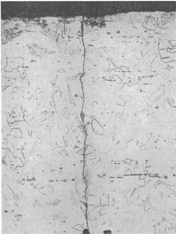
FIG. A.—Nail A.49. Transcrystalline crack parallel to fracture. ( \times 200 .)
