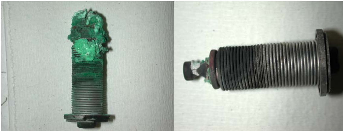
Fig. 4. Bellows C (left) and D (right) at the end of testing (28 days).
