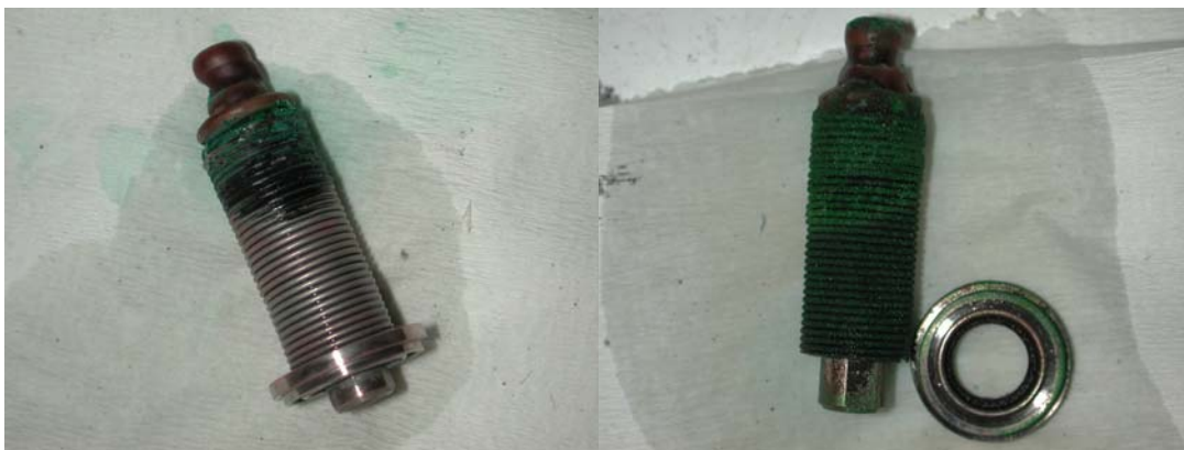
Fig. 6. Comparison of bellows A (left) and B (right) after 32 h of HF exposure.
