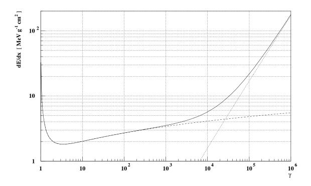
Figure 3.1: Energy loss of muons in air as function of Lorentz factor. The contributions from ionization (dashed line) and direct pair production (dotted line) are indicated.
