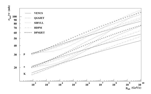
Figure 4.3: Inelastic cross sections of protons, pions, and kaons with protons for the models used in CORSIKA as function of projectile momentum. For HDPM see footnote in Appendix C.
