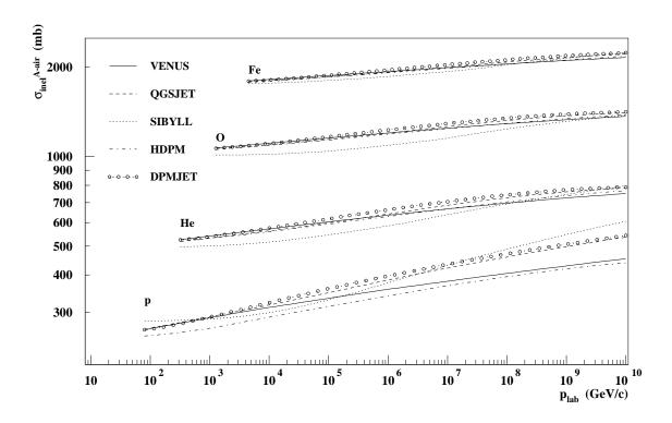
Figure 4.4: Inelastic nucleus-air cross sections of various projectile nuclei for the models used in CORSIKA as function of projectile momentum. For HDPM see footnote in Appendix C.
