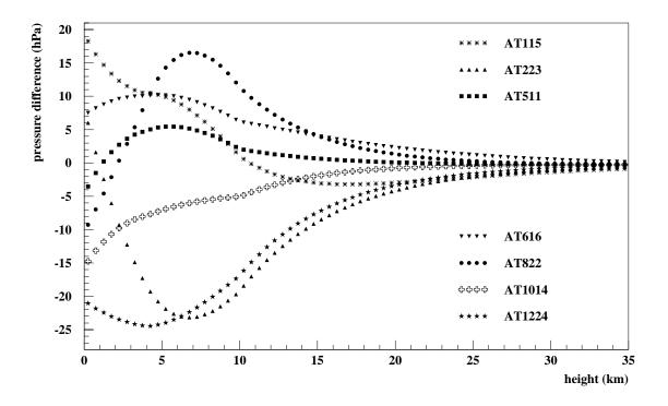
Figure 2.1: Pressure difference of the atmosphere above Stuttgart (Germany) at 7 days distributed over the year 1993 relativ to U.S. standard atmosphere.
