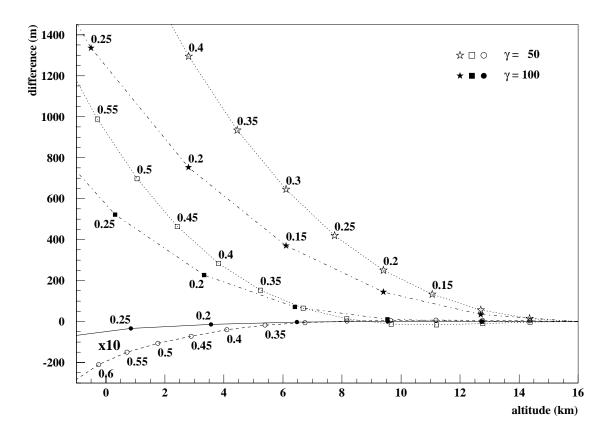
Figure B.1: Differences in the muon range calculated for vertical muons of  $\gamma = 50$  (open symbols) and 100 (filled symbols) starting at 16 km altitude. The difference to the real penetration depth is shown for different approximations:  $\star$  Equation 4.2, Equation B.2, and  $\bullet$  (with x10 enlarged scale) Equation 4.5. The numbers give the fraction of the mean life time in the muon rest system.
