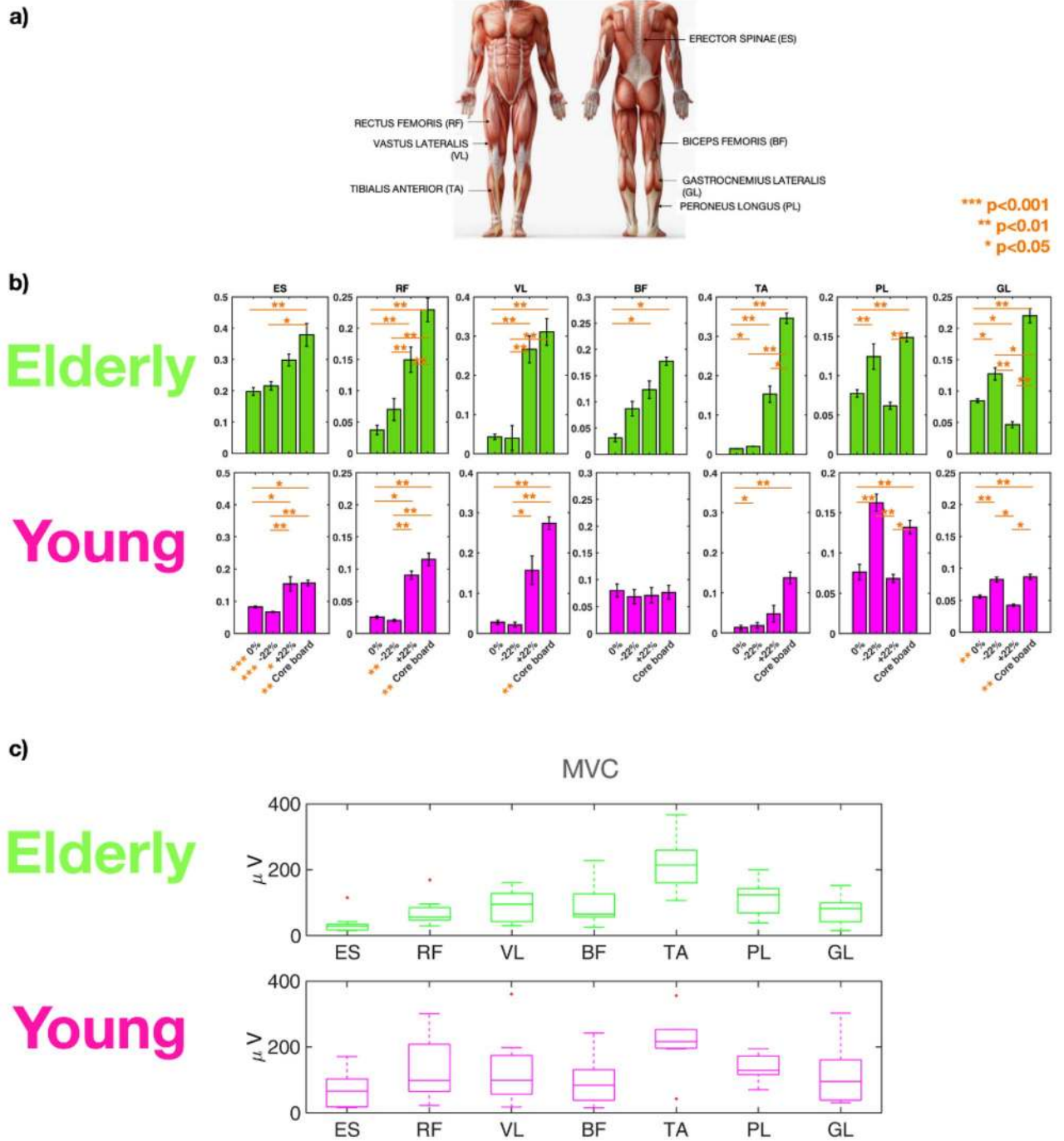
Figure 7. (a) Muscle activity as measured using EMG sensors. (b) RMS EMG results. Median values across the elderly (in green) and the younger adults (in pink) of the RMS values for each muscle (ordered in column): Erector Spinae (ES), Rectus Femoris (RF), Vastus Lateralis (VL), Biceps Femoris (BF), Tibialis Anterior (TA), Peroneus Longus (PL) and Gastrocnemius Lateral head (GL) in static (0%, ± 22%) and dynamic (core board) conditions. P-values are represented by asterisks. In each box, p-values represent statistically significant differences among postural conditions within the same group. P-values reported in the x-axis represent statistically significant differences between the two groups under the same postural conditions. (c) MVC results. Boxplots display the maximum voluntary contraction values for the elderly (in green) and for the younger adults (in pink).
