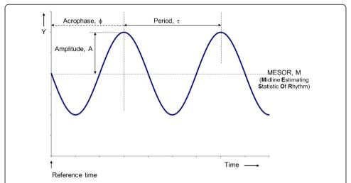
**Figure 1 Definition of rhythm characteristics.** The MESOR is a rhythm-adjusted mean; the double amplitude (2A) is a measure of the extent of predictable change within a cycle; the acrophase is a measure of the timing of overall high values recurring in each cycle, expressed in (negative) degrees in relation to a reference time set to 0°, with 360° equated to the period; and the period is the duration of one cycle. © Halberg Chronobiology Center.
