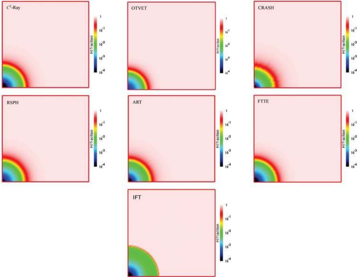
Figure 11. Test 2 (H II region expansion in a uniform gas with varying temperature): images of the H I fraction, cut through the simulation volume at coordinate z = 0 at time t = 10 Myr for (left to right and top to bottom) C^2 -RAY, OTVET, CRASH, RSPH, ART, FTTE and IFT.
