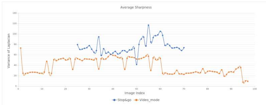
Figure 2. Image sharpness comparison between stop&go dataset and video_mode dataset using Variance of Laplacian
