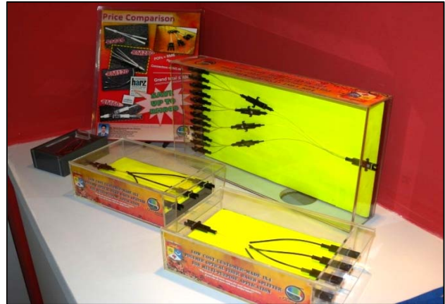
Figure 4 Final product of 1x12 POF based optical splitter and also 1x3 and 1x4 splitters
