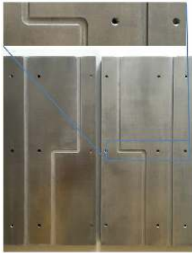
Fig. 13: Integrated circuit for verifying the performance of straight and double 90° bent waveguide lines. There is no EBG structure at the location of the junction.
