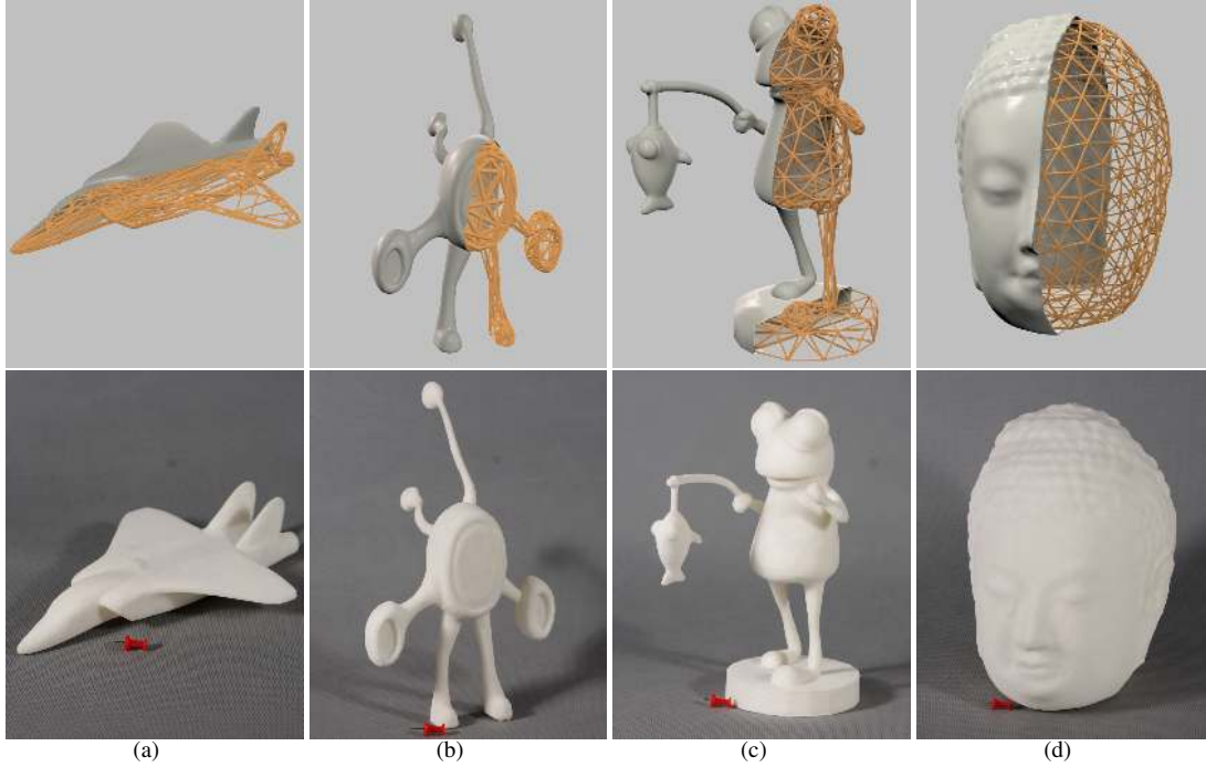
Figure 8: Printed objects using powder-type printers (P-1) produced by our algorithm. From left to right: Fighter, TV-Alien, Fishing-Frog, and Buddha-Head. The upper row shows the rendering results with half skin and half frame. The lower row shows photos of the printed objects. The largest edge length of the bounding box of each object is 200mm. A small red drawing pin is put beside each object as a size reference.
