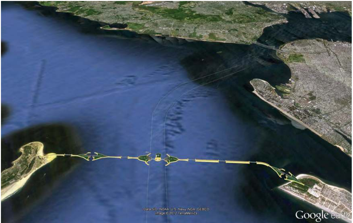
Figure 4.12. Plan showing the extent of the causeway and berms forming the gateway barrier (adapted from Padron and Forsyth, 2009).
