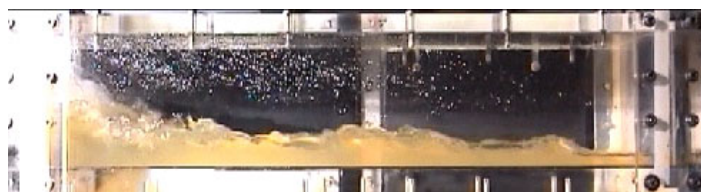
e) The liquid film depth thins progressively. This effect is much more important at the end of the test section than at the beginning.
