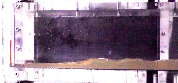
Fig. 4.9. Occurrence of a hydraulic jump at the beginning of the test section.
