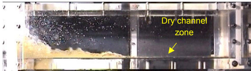
Fig. 4.15. Totally reversed flow with dry channel zone.
