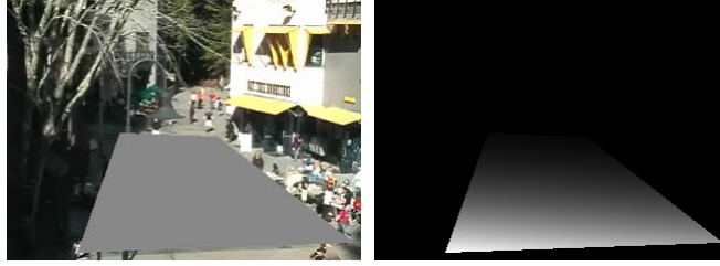
Figure 5: Density estimation. Left: region of interest in the image. Right: density map (weights).
