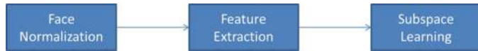
Fig. 2. Three stages in face recognition based on the framework of local features and subspace learning.
