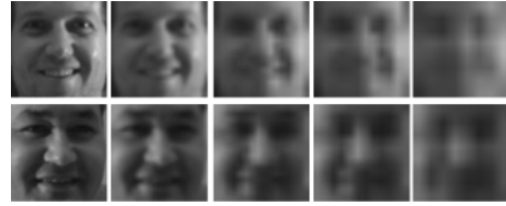
Fig. 8. Cropped face image examples for three subjects. From left to right: high resolution ( 32 \times 32 ), followed by low resolution ( 16 \times 16 , 8 \times 8 , 6 \times 6 , 4 \times 4 ) images.
