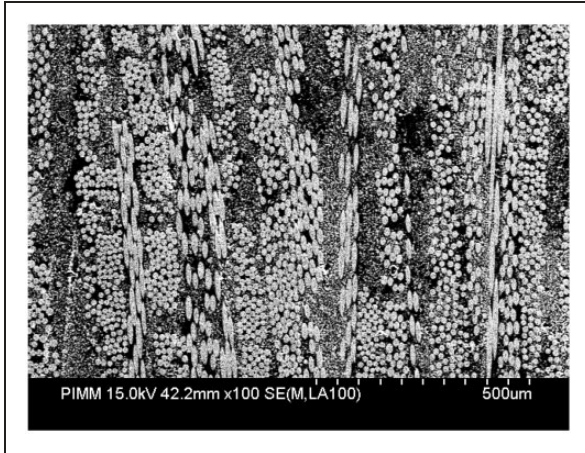
Figure 1. Typical microstructure of A-SMC observed by mean of a SEM: randomly oriented bundle of fibers.
