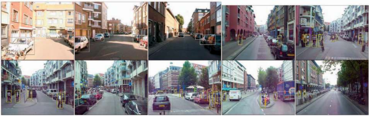
Fig. 14. Example car and pedestrian detections of our system on difficult images from the two test sequences.
