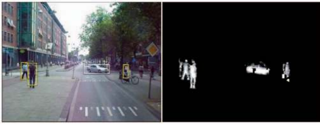
Fig. 5. Detections and corresponding top-down segmentations used to learn the object-specific color model.
