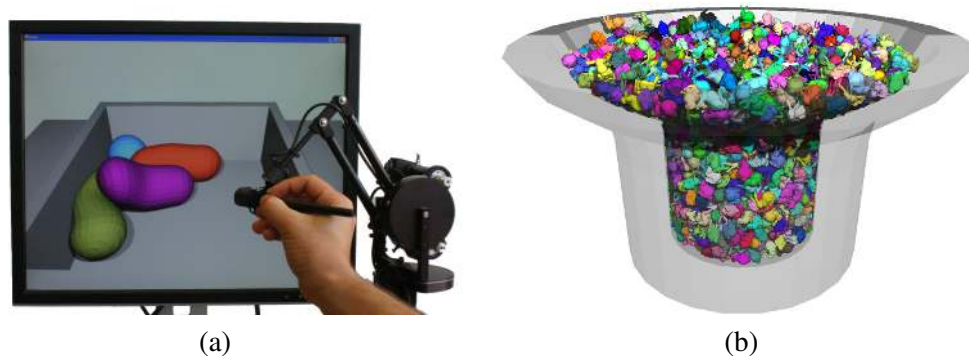
Figure 7.9: (a): A \sim 100 Hz, force-feedback, haptic simulation of deformable and rigid frictional contact using Staggered Projections. (b): A preliminary decomposition approach as validated on a high-dimensional, high-contact count scene, composed of two-thousand rigid-body models.
