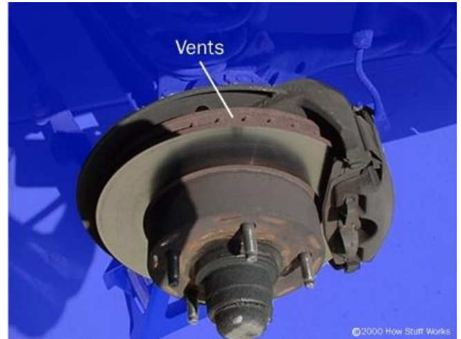
Fig -2: Vents provided on Disc Brakes
