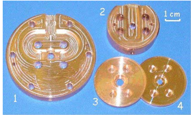
Figure 5. General view of the double (1) and single-feed (2) mode launchers together with matching (3) and regular (4) cells.
