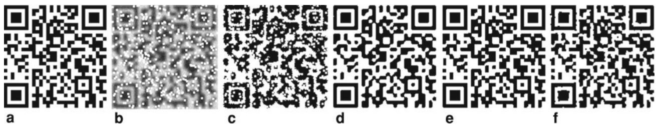
Fig. 5 Segmentation of a noisy, blurred QR code with missing data. (a) QR code of the GLM wikipedia page URL. (b) Noisy (Gaussian noise, SNR = 16), blurred (Gaussian blur, standard deviation 2 pixels) QR code with 16 % randomly missing pixels. (c) Otsu thresholding of (b). (d–f) ASBS results for a two-region segmentation/deconvolution
