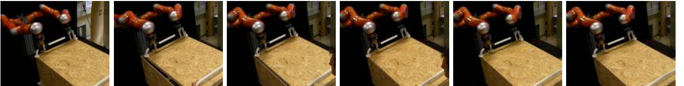
Fig. 11. The position of the box, lid, and the robots in the demonstration in the leftmost picture. Positions after each epoch, with epoch number increasing towards the right. Only 5 epochs are shown because the pictures of the final position after epoch 5 are practically identical.
