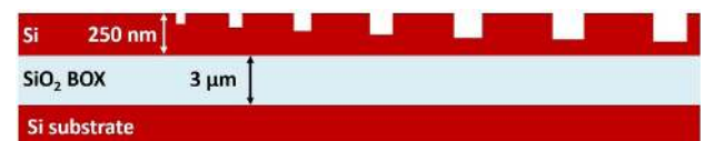
Fig. 36. Schematic representation of the multi-etch GC proposed in [81], where the lag effect of ICP-RIE is exploited.
