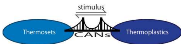
Fig. 1 Covalent adaptable networks (CANs) exhibit many of the properties of thermosets, while also possessing the triggerable processability and relaxation behavior of thermoplastics. CANs represent a unique class of materials that not only combine the desirable behaviors of each of these materials, but also enable the transition from one set of material properties ( i.e. , thermoset-like) to the other ( i.e. , thermoplastic-like) either upon application of an external stimulus, such as light or temperature, or simply by considering the material behavior on different timescales that are intimately linked to the timescales of network rearrangement.
