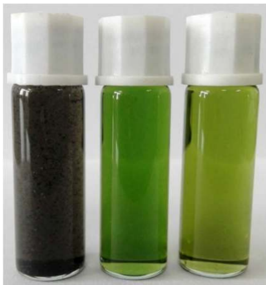
Figure 2. Photographic image of the samples' dispersion in DMSO (left to right: RGO, RGO-TPP 1, and RGO-TPP 2).
