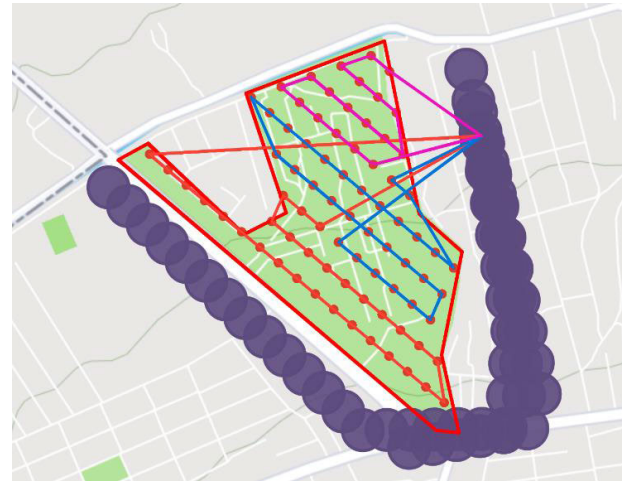
FIGURE 7. Route of the flyby of the "Complex" field with the movement of the vehicle. Different colors of the lines indicate separate take-off and landing cycles.
