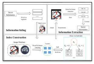
Fig. 8. The proposed CIS (Q. Liu, X. Xiang, J. Qin, Y. Tan, Y. J. E. J. o. I. Qiu, et al., 2020).
