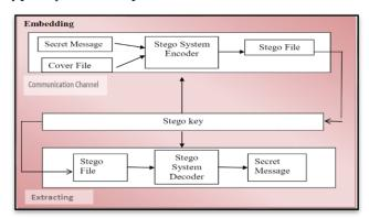
Fig. 1. General model of Steganography (OMRAN et al., 2022).
