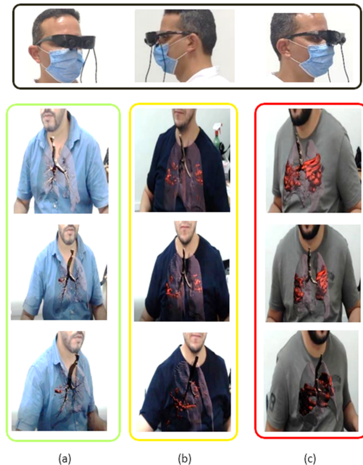
Figure 5. Augmented reality viewer with different stages of disease severity with different patients, (a) mild, (b) moderate and (c) critical infection.
