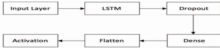
Figure 3. Long Short-Term Memory network architecture
