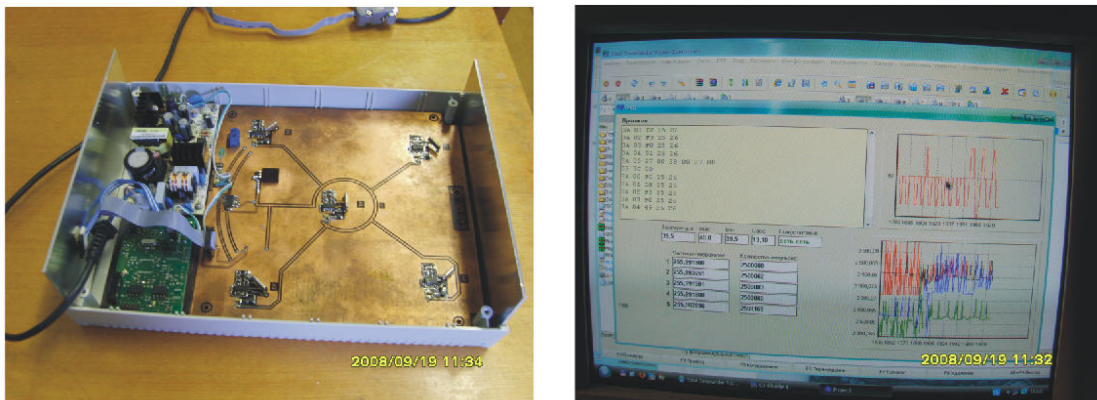
Figure 6. The appearance of the dosimeter (with the cover removed)
