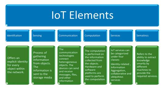
Figure 1. Main elements of an IoT system [9].
