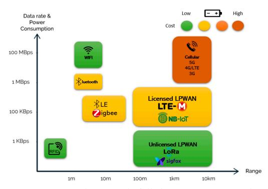
Figure 4. Communication techniques in IoT classified by data rate, power consumption, and range.
