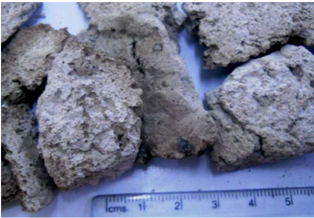
Fig. 2 Image of precipitated dried struvite taken with Nikon COOLPIX L21 digital camera
