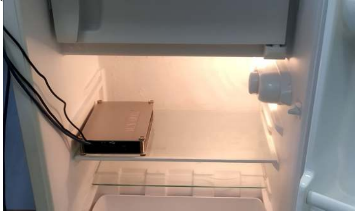
Figure 6: Picture of one of the four boards encapsulated in a metal case inside an ordinary household refrigerator. Three cables coming out of the case are USB, Ethernet, and Power.
