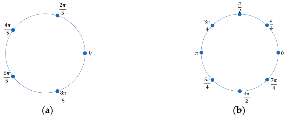
Figure 2. Constellation example for a binary CPM (a) h = 2/5 (b) h = 1/4 .
