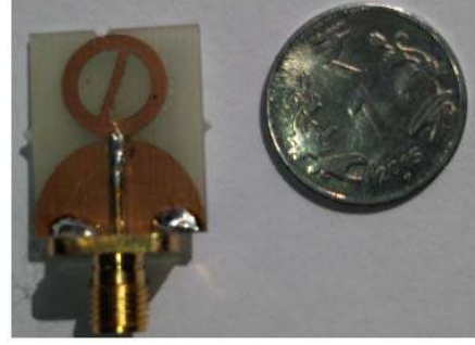
Figure 4. Prototype of the designed antenna.
