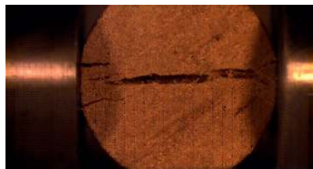
FIGURE 3: Destruction process images for rock specimen under SHPB impact damage.
