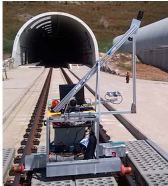
Figure 5. Prototype of the tunnel inspection platform.
