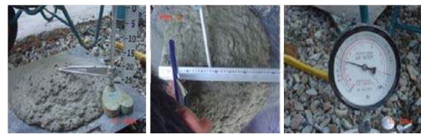
Fig. 21 Initial workability test of fabricated self-healing concrete (Target : slump 21cm, slump flow around 40 cm x 40 cm, Air 4.5%).
