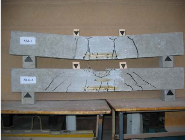
Fig 12. Crack pattern of control SK6 beams
