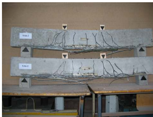
Fig 10. Crack pattern of SA6 series beams
