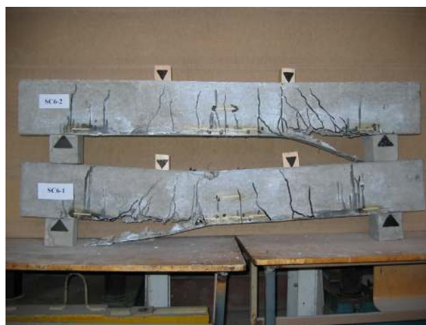
Fig 11. Crack pattern of SC6 series beams
