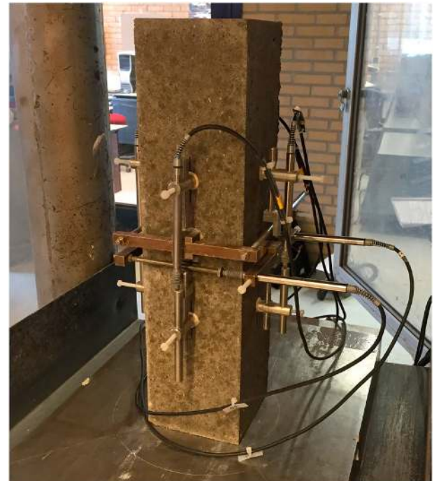
Fig. 1. Testing set-up for elastic modulus measurement on AAC.
