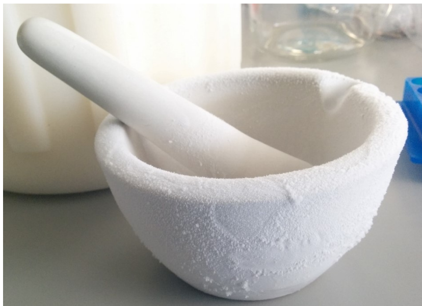
Figure 23: Hand mortar and pestle used to crush DNA of fungi with liquid nitrogen
