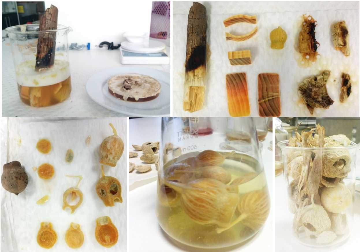
Figure 8: Wood and gumnut slices soaked in hydrogen peroxide solution for the second step of the transparent wood protocol and left to dry
