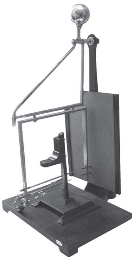
Figure 4. Broca’s stereograph (Collection of scientific instruments, Biological Anthropology Sector, Museu Nacional/ UFRJ)
