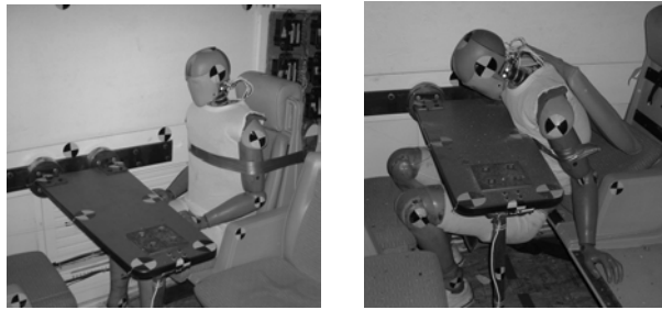
Figure 9 – THOR ATD before (left) and after (right) two-car full-scale test
