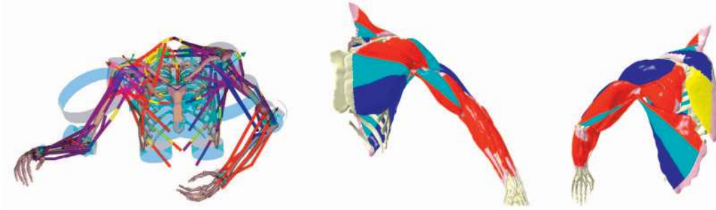
Fig. 4. The leftmost figure shows the piecewise linear muscle models with wrapping surfaces to model muscle contact in inverse dynamics calculations. Larger muscles have multiple contractile regions with individual activations and these must be embedded in the tetrahedron meshes for simulation (rightmost figures).
