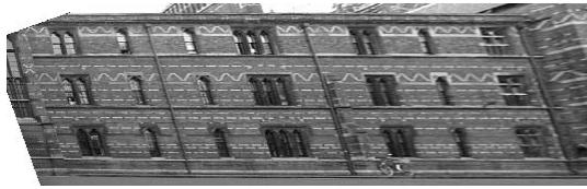
Figure 5: The affine rectified image. Notice that parallelism is restored, but angles and ratios of lengths are still incorrect.
