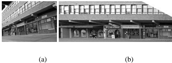
Figure 11: Plane rectification via partial internal parameters. (a) Original image. (b) Rectification where the relative scaling of vertical and horizontal directions assumes a natural camera with the principal point at the centre of the image. The focal length is computed from the single orthogonal vanishing point pair. Measurement of the aspect ratio of a window indicates a difference of 3.7% between true and computed values. Note that the two parallel planes, the upper building facade and the lower shopfront, are both correctly rectified, but scene planes not parallel to these two are distorted by the rectification homography. This distortion is visible on the area of overhang of the upper facade.
