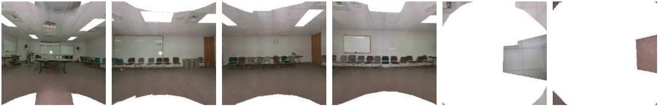
Figure 5: Cubical texture-mapped model of conference room (from 75 images taken with a hand-held digital camera).
