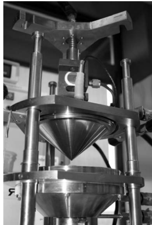
Fig. 3 Shearing device used for processing concentrated biopolymer systems. The diameter of the upper cone is 12 cm. The cone angle is 100^\circ , the angles between the cones are 2.5^\circ . The rotational speed can be varied from 5 to 250 rpm, leading to a shear rate ranging from 12 to 600\text{ s}^{-1} . The maximum shear stress that can be applied is 40 kPa. The system is temperature controlled through an external water bath. More details can be found in Peighambardoust et al. 19,23 and Manski et al. 24
