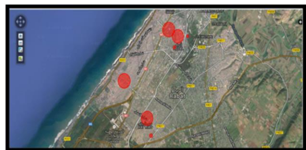
Figure 8: Image Satellite Displaying data : areas of the red dots representing each BTS is proportional to the annual traffic intensity recorded for each of the BTS
